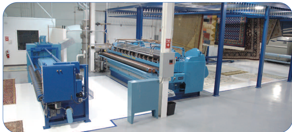
Modern rug plants often speed up production with an automated washer with a compression wringer followed by hanging rugs on a dry tower.
