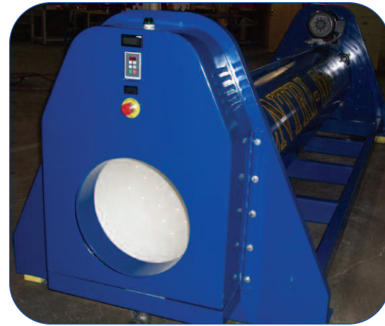
European rug cleaning companies have been using centrifuge technology for years. The centrifuge used in a modern rug plant saves space, money and speeds up the drying process for rugs.
